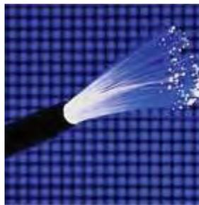
Exhibit JPL-4, reproduced above, depicts the fiber optic strands inside a cable of the nature used by TWC. When TWC transmits additional bits over its fiber to add a new video channel, broadband bandwidth or voice service, there is no physical impact on the pole attachment. In other words, lighting a strand of fiber to add a service does not affect the actual fiber cable that is attached to the pole.
